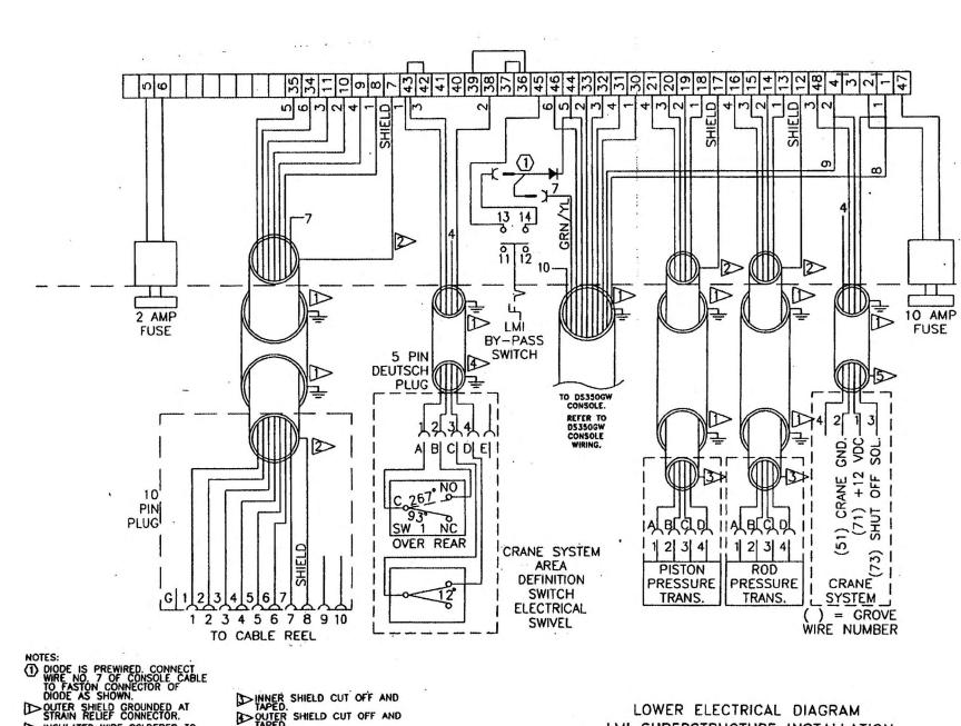
INSULATED WIRE SOLDERED TO INNER SHIELD AND CONNECTED AS SHOWN.
